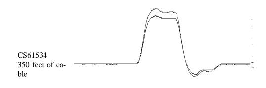
Figure 8 - Mistermination and gain error can have significant effect on pulse amplitude. The larger pulse results from the use of probes which are not well matched,
