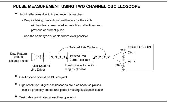
Figure 7 - Recommended pulse shape measurement test configuration and guidelines.
