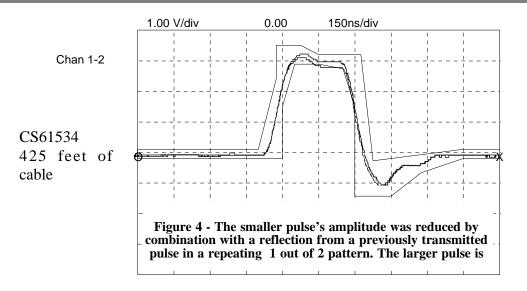
flections. In order to avoid reflections in a transmission line, impedance mismatches should be avoided, and the line should be terminated with a load that is equal to the characteristic impedance of the line. Proper terminations are every bit as important when measuring pulses in the lab as they are in connecting up the network.
