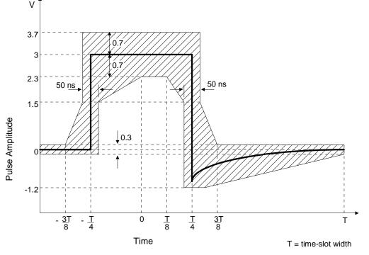
Figure 3 - CCITT Rec. G.703 pulse shape for 1.544 MHz operaton.
